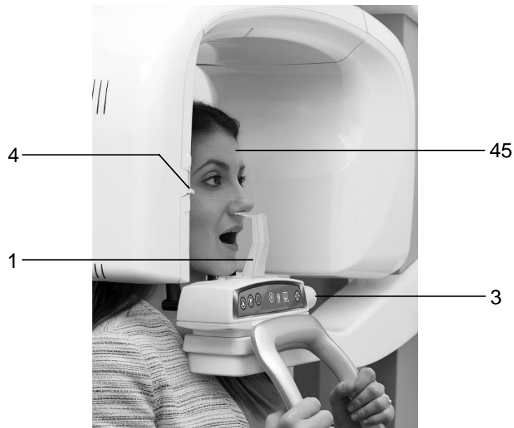
Figure 32: 2D TMJ closed mouth patient positioning
